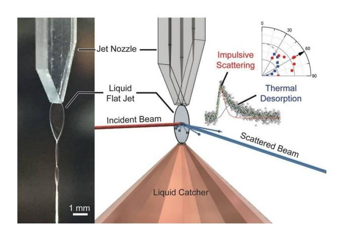
Left: a liquid dodecane flat jet produced by a microfluidic chip nozzle. Right: an incident molecular beam (red line) striking the jet surface. Researchers can analyze the velocity and angular distributions of molecules in the scattered beam (blue line). Credit: Chin Lee, University of California at Berkeley
