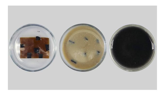
Two different PDK plastics in acidic solution, demonstrating how each polymer easily breaks down into individual monomers in different steps conducted at different temperatures, which allows for complete recycling of both plastics. Credit: Jérémy Demarteau/Berkeley Lab
