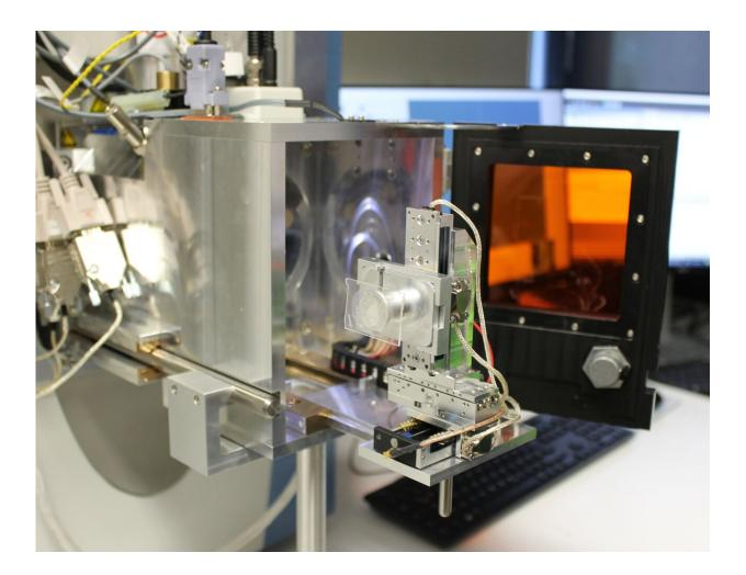
A sample is clamped in the traverse table of the ionization chamber. Credit: UBT / Chr. Wißler.
