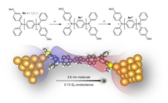
Top: the two-step oxidation of the bis(triarylamines) molecular series. Bottom: the geometry of the highest conducting trimer (n=3) molecule in the molecular junction. Red and blue regions are artistic depictions on the coupling between the two edge states. Credit: Liang Li/Columbia University
