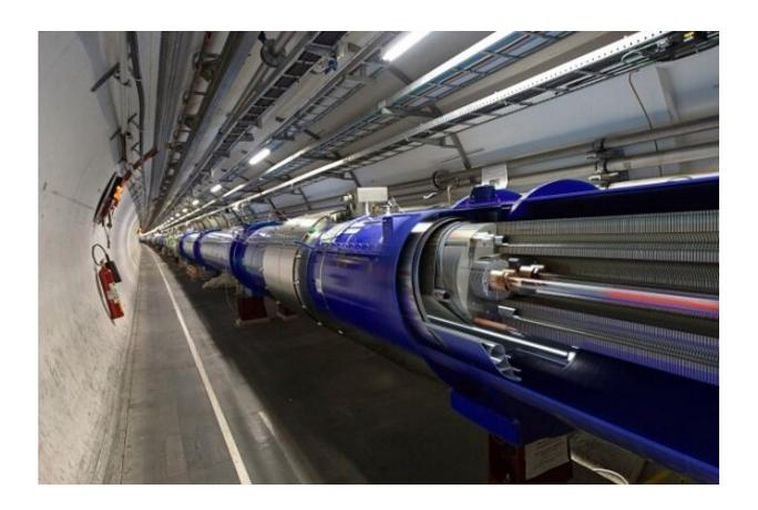
3D cut of the LHC dipole. Credit: CERN
