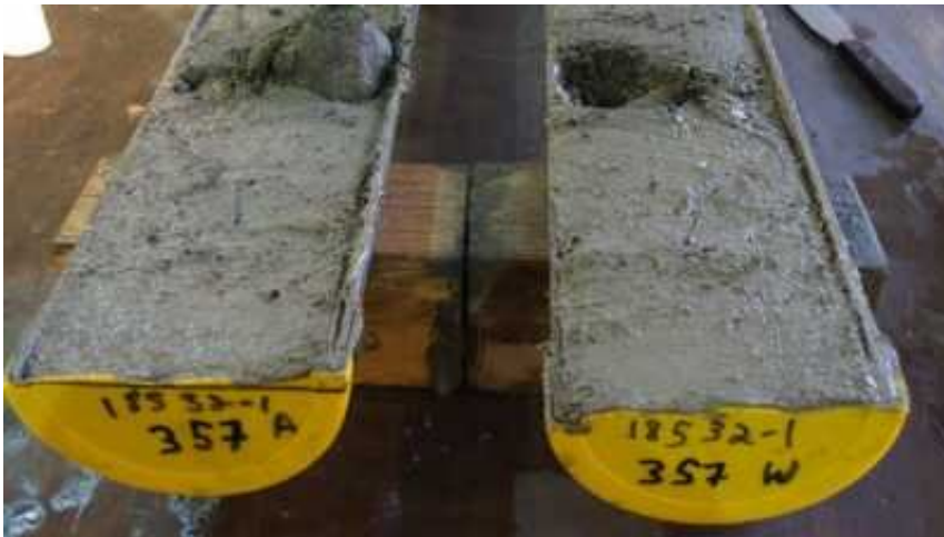
Deep sea sediment core with coarse ice-transported lithogenic components (Heinrich layer). Credit: Lars Max
