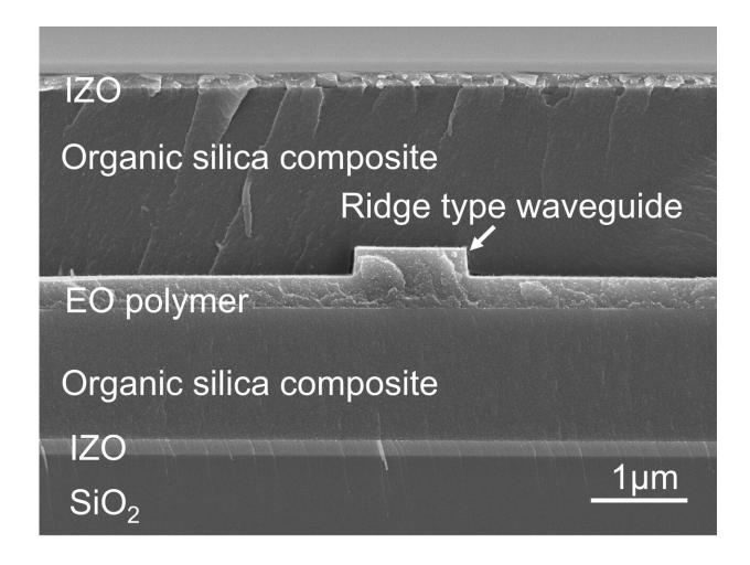
Cross section of EO polymer optical modulator for visible light. IZO (Indium Zinc Oxide) electrode are placed at the top and bottom of waveguide. Credit: National Institute of Information and Communications Technology (NICT)
