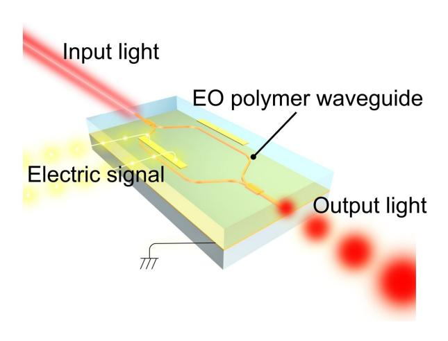
Schematic diagram of EO polymer optical modulator for visible light. The input light propagates through the EO polymer waveguide, and an output optical signal corresponding to the electric signal is output. Credit: National Institute of Information and Communications Technology (NICT)
