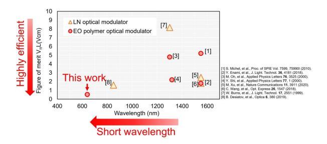
Relationship between operation wavelength and figure of merit of optical modulator. (This work and previous LN and EO polymer optical modulator.) Credit: National Institute of Information and Communications Technology (NICT)
