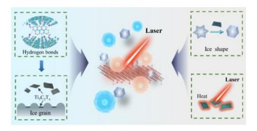
Synergetic ice inhibition effects of two-dimensional  $Ti_3C_2T_x$  MXene nanosheet. Credit: CAO Yuan et al.
