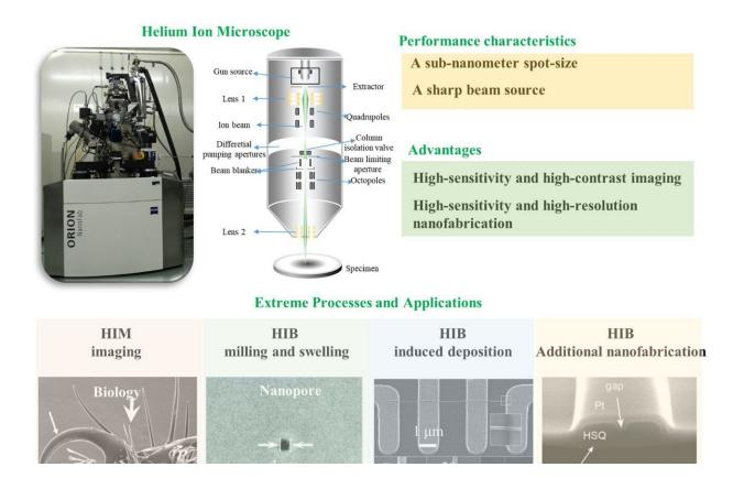
Providing a helium ion microscope system with GFIS that can be used for extreme nanostructures fabrications with high resolution and sensitivity. Credit: Shixuan He et al
