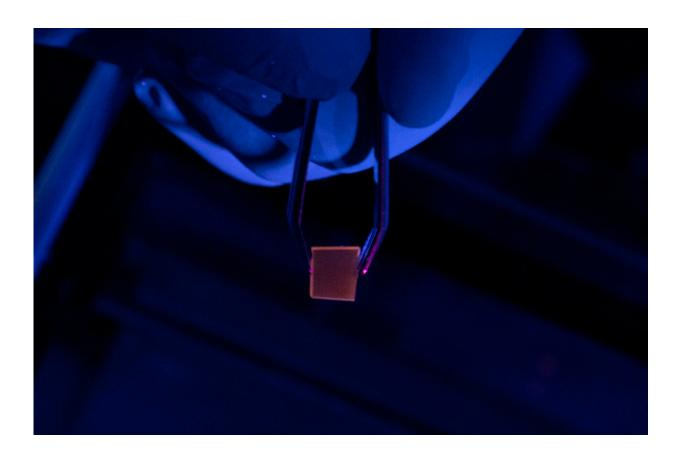
Researchers created a new glass-ceramic that emits light in response to mechanical stress. The highly transparent material is made from a potassium germanate glass matrix embedded with chromium-doped zinc gallate (ZGO) crystals that give the material its mechanoluminescent properties. Credit: Lothar Wondraczek, Friedrich Schiller University Jena
