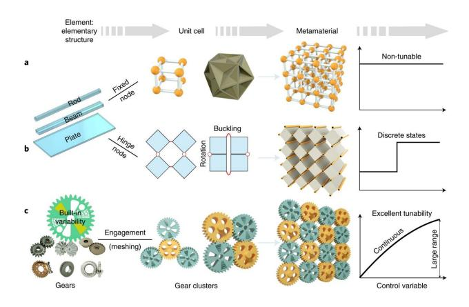
Design concepts of mechanical metamaterials. a,b, Classical paradigm: nontunable metamaterial (a) and typical reconfigurable metamaterial (b). c, Gearbased metamaterials. Credit: Nature Materials (2022). DOI: 10.1038/s41563-022-01269-3
