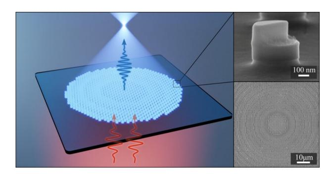
An array of several hundred chair-shaped nanostructures (on the right in an electron-microscope picture) is able to halve the wavelength of an incident "red" beam and focus the generated "blue" beam at a desired distance. Credit: Compuscript Ltd
