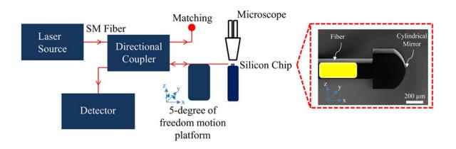
Silicon micromirrors coupling efficiency measurements using single-mode optical fibers fed from monochromatic light source, a directional coupler and an optical detector. Credit: Yasser M. Sabry et al, *Journal of Optical Microsystems* (2022). DOI 10.1117/1.JOM.2.3.034001
