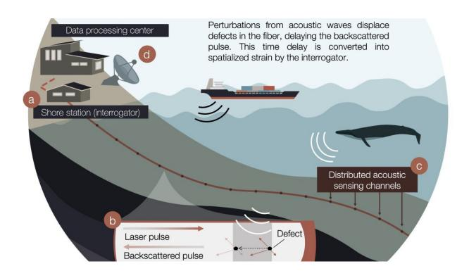
The illustration shows how DAS works. An interrogator (a) sends a laser pulse from a ground station through the fiber optic cable. The cable has defects (b) which underwater sounds slightly displace. This sends back a signal that the interrogator can interpret as acoustic data over regularly spaced intervals or channels (c). Credit: Marte Finsmyr and Léa Bouffaut
