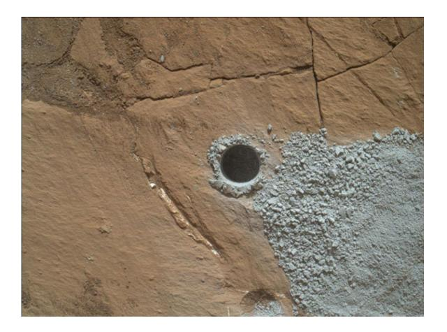
NASA's Curiosity Mars Rover drilled this hole to collect sample material from a rock target called "Buckskin" on July 30, 2015. The diameter of the hole is slightly smaller than a U.S. dime. Rock powder from the drill site was subsequently delivered to a laboratory inside the rover and found to contain the rare mineral tridymite. Credit: NASA/JPL-Caltech/MSSS
