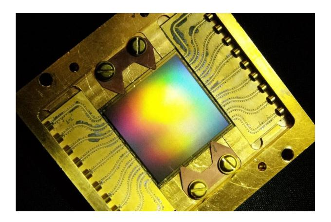
The sensor mounted for use in an MKID Exoplanet Camera. Credit: Ben Mazin
