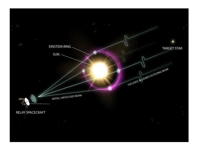
Communications across interstellar distances could take advantage of a star's ability to focus and magnify communication signals through an effect called gravitational lensing. A signal from—or passing through—a relay probe would bend due to gravity as it passes by the star. The warped space around the object acts somewhat like a lens of a telescope, focusing and magnifying the light. A new study by researchers at Penn State investigated our solar system for
