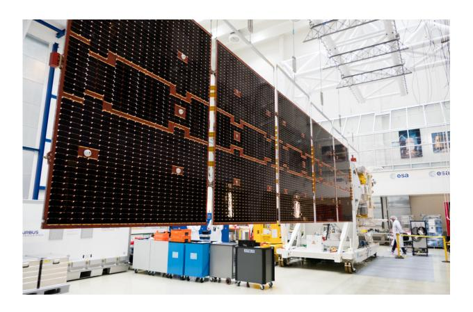
EarthCARE solar wing deployed. Credit: ESA-M. Cowan, CC BY-SA 3.0 IGO
