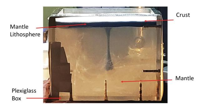
A simulation of the rocky outermost layer of Earth's shell using silicone polymer fluid, modeling clay, and a sand-like layer made from ceramic and silica spheres demonstrates the process of lithospheric dripping. Credit: Julia Andersen/Tectonophysics Lab/University of Toronto
