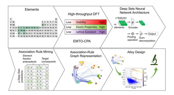
Shown is a data-driven workflow to map the elastic properties of the highentropy alloy space. Credit: Chen et al.
