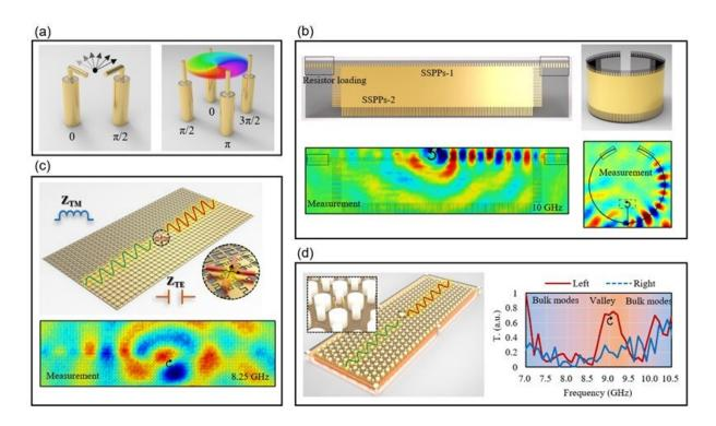
Unidirectional excitation of various metamaterial interface waveguides. (a) Sources with the angular momentum. (b) SSPPs ( $\pm\epsilon$ eff). (c) LWs ( $\pm$ Zsurf). (d) Valley PTIs ( $\pm\Phi$ Berry). Credit: Xu et al., DOI: 10.1117/1.AP.4.4.046004
