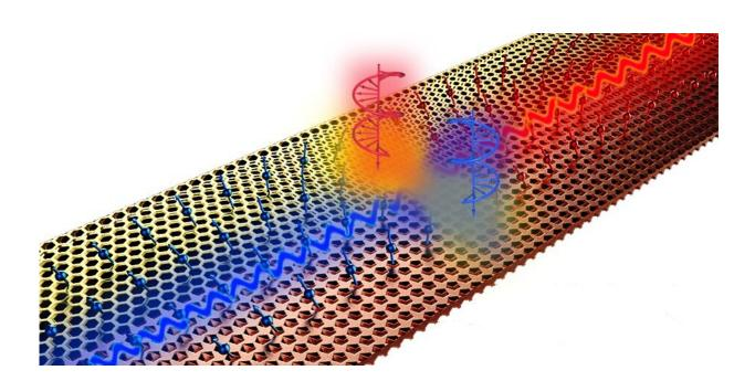
Unidirectional excitation of metamaterial interface waveguides; the chirality of the source decides the direction of energy flow along the edge. Credit: Zhixia Xu
