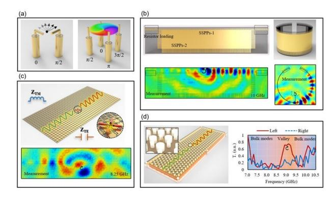
Unidirectional excitation of various metamaterial interface waveguides. (a) Sources with the angular momentum. (b) SSPPs (±εeff). (c) LWs (±Zsurf). (d) Valley PTIs (±ΦBerry). Credit: Xu et al., DOI: 10.1117/1.AP.4.4.046004
