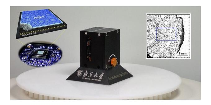
A chip-scale metalens array makes this microscope system ultracompact. Credit: Tao Li, Nanjing University.
