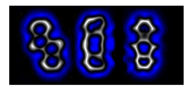
Images of single molecules obtained by high-resolution atomic force microscopy. Selectively and reversibly the molecular structure in the center can be transformed to the structure on the right or on the left, by voltage pulses applied form the tip of a scanning probe microscope. Credit: Leo Gross/IBM
