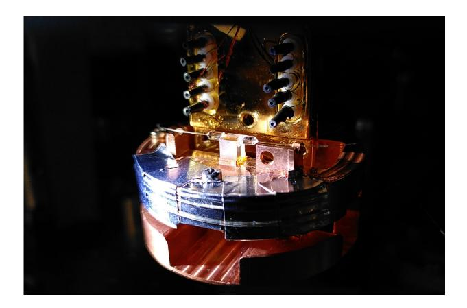
Picture of the quantum memory attached to the optical fiber. Credit: ICFO/ S. Grandi
