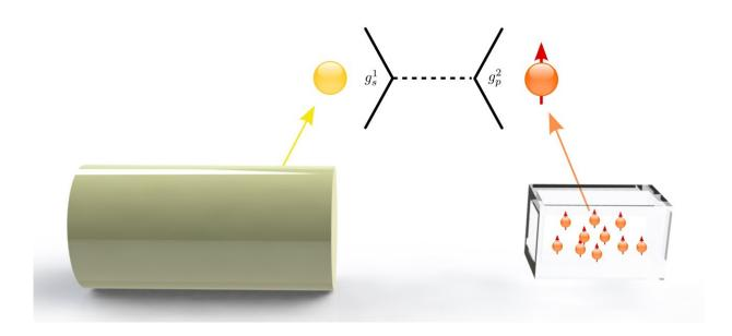
Schema of a co-magnetometer. The right is a cell containing atoms, and the left is a nearby mass. Credit: SHENG Dong and LU Zhengtian's team
