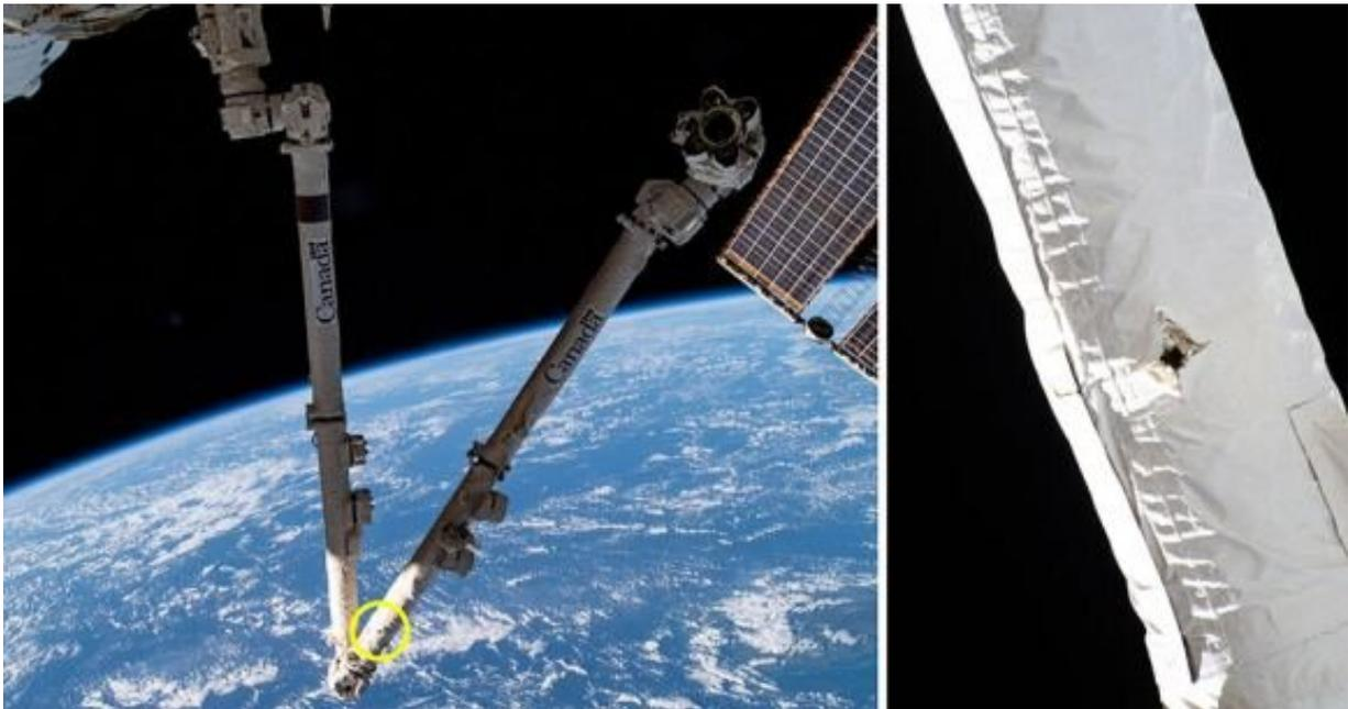
Photograph of Canadaarm2 hit by a piece of space debris. Credit: NASA
