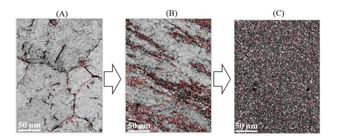
Images of aluminum alloy 7075 taken with a scanning electron microscope before (A), during (B), and after (C) going through the ShAPE machine show how the microstructure of the alloy changes dramatically during extrusion. The shearing effect of the ShAPE machine breaks up particles, which are akin to lumps in cake batter, into much smaller pieces to create a more uniform microstructure. Credit: Image by Joshua Silverstein | Pacific Northwest National Laboratory
