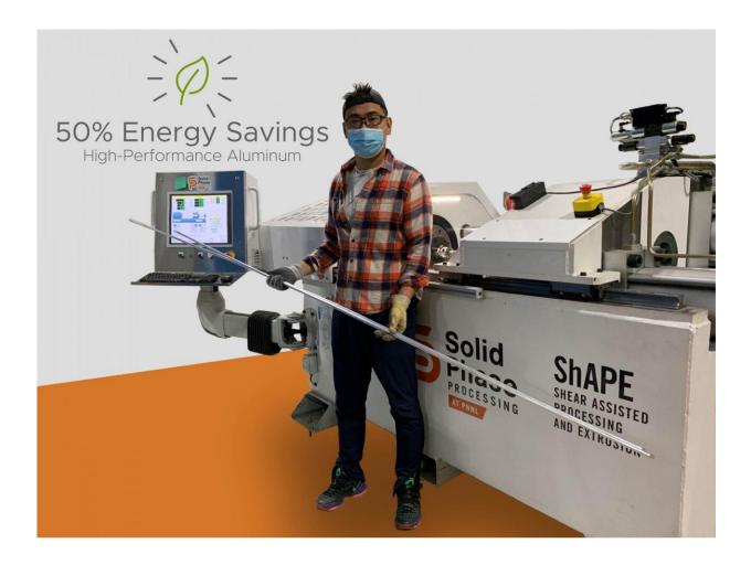
Shear Assisted Processing and Extrusion (ShAPE<sup>TM</sup>), developed by researchers at Pacific Northwest National Laboratory, improves the energy efficiency of producing extruded high-performance aluminum alloys. Credit: Composite image by Cortland Johnson | Pacific Northwest National Laboratory
