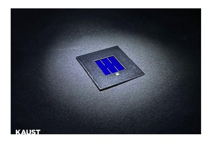
Considerable performance gains in perovskite-silicon tandem solar cells (such as that pictured above) can be achieved by adding a magnesium fluoride interlayer. Credit: 2022 KAUST; Erkan Aydin
