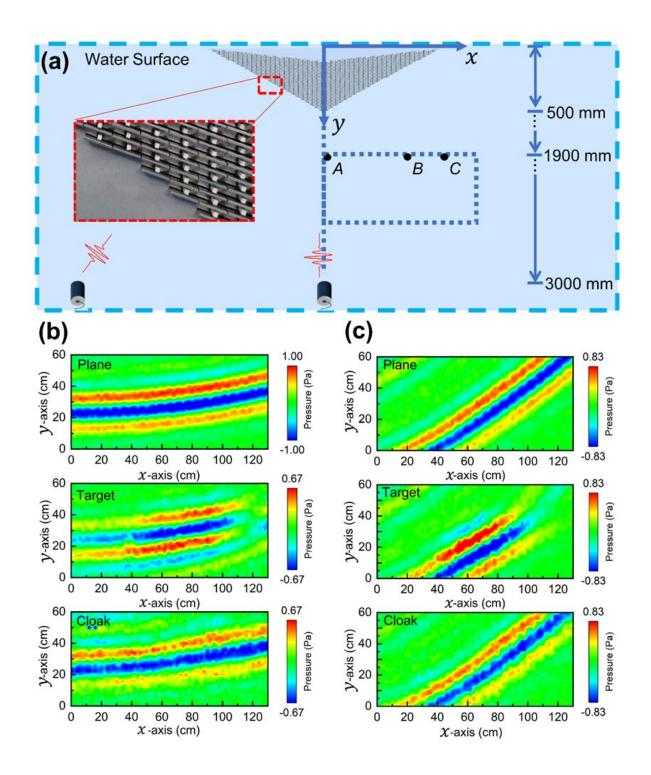
Fig. 2 Experimental demonstration of the underwater acoustic carpet cloak. Credit: IACAS
