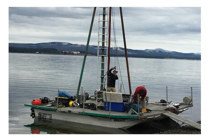
Coring platform at Yellowstone Lake. The long metal tubes are coring barrels used to collect cores. Credit: Lisa Morgan
