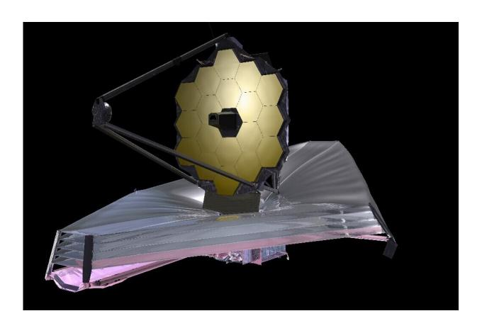
A wonder of engineering, Webb is able to gaze further into the cosmos than any telescope before it thanks to its enormous primary mirror and its instruments that focus on infrared, allowing it peer through dust and gas.
