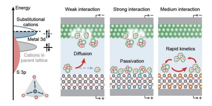
Schematic diagram of design principles for high-efficient lithium-sulfur catalysts. Credit: Shen Zihan
