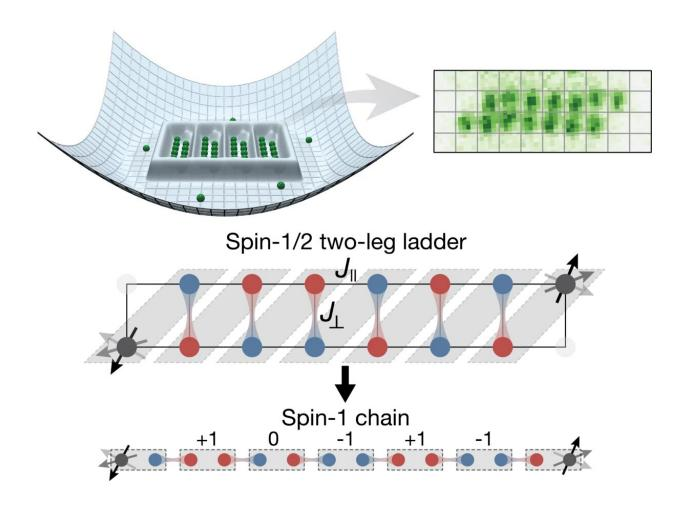
Illustration of the main concepts in the paper: on the left an illustration of the lattice potential used, on the right an exemplary snapshot of a single ladder with 14 individual atoms visible in green. Below that, a schematic explanation of how the ladder geometry is mapped onto a spin-1 chain. The dangling edge spins are shown in grey. Credit: Max Planck Society
