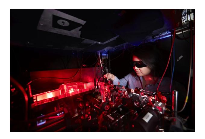
Dr Pimonpan Sompet (first author of the paper) aligning the second-harmonic generation cavity. The researchers use the UV light produced in here to cool the lithium atoms in the experiment. Credit: MPQ
