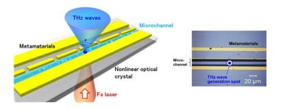
Fig.1 Schematic diagram and photograph of the newly developed terahertz (THz) biochemical chip. The chip is made of GaAs, a nonlinear optical crystal, and is composed of five metamaterial units and a single microchannel on the surface. By irradiating with a femtosecond laser from the back surface of the crystal, a point THz light source is generated to interact with the solution. Credit: Kazunori Serita
