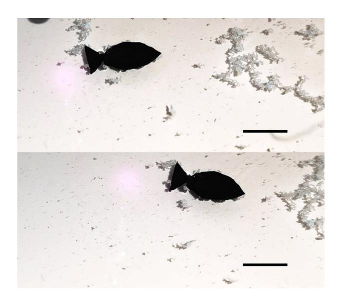
A light-activated fish-shaped robot collects microplastics as it swims (scale bar is 10 mm). Credit: Adapted from *Nano Letters* 2022, DOI: 10.1021/acs.nanolett.2c01375
