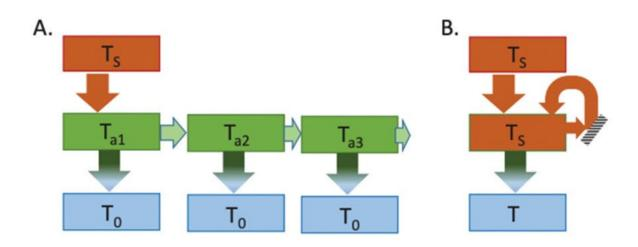
Unlike a multiphotovoltaic cell system where the emitted light is absorbed by a subsequent cell (left), the single cell nonreciprocal photovoltaic converter proposed by Sergeev and Sablon (right) causes emitted light is re-absorbed by the same cell, limiting emission losses without the need for additional PV cells. Credit: Sergeev and Sablon, *Journal of Photonics for Energy* (2022) DOI: 10.1117/1.JPE.12.032207.
