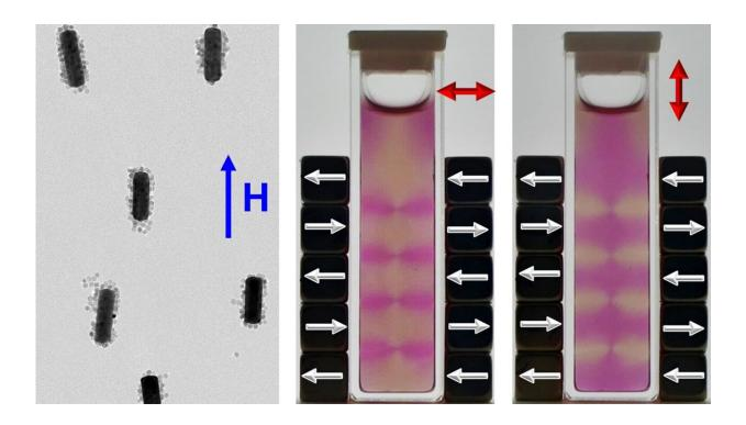
Electron micrograph of gold nanorods overcoated with iron oxide nanoparticles and aligned in a magnetic field. Credit: Mehedi H. Rizvi
