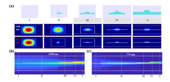
(a) The simulated distribution of TE00 modes of 1550 nm and 775 nm at different cross sections of the coupler; simulated mode propagation in the designed coupler at wavelengths (b) 1550 nm and (c) 775 nm. Credit: Liu et al., *Advanced Photonics Nexus* (2022). DOI 10.1117/1.APN.1.1.016001.
