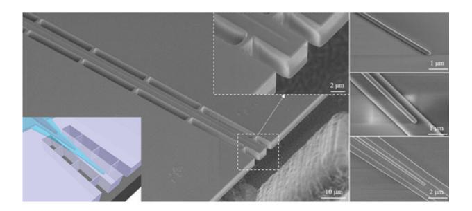
Three-dimensional structure of the X-cut edge coupler, consisting of a suspended SiO2 waveguide and a tri-layer SSC. Credit: Liu et al., *Advanced Photonics Nexus* (2022). DOI 10.1117/1.APN.1.1.016001
