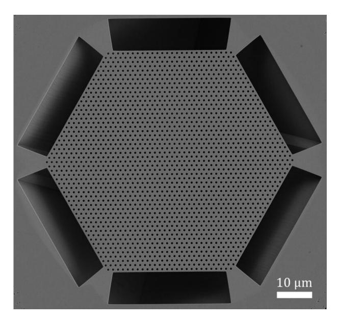
Top view of a scanning electron micrograph of the Berkeley Surface Emitting Laser (BerkSEL). The hexagonal lattice photonic crystal (PhC) forms an electromagnetic cavity. Credit: the Boubacar Kanté group
