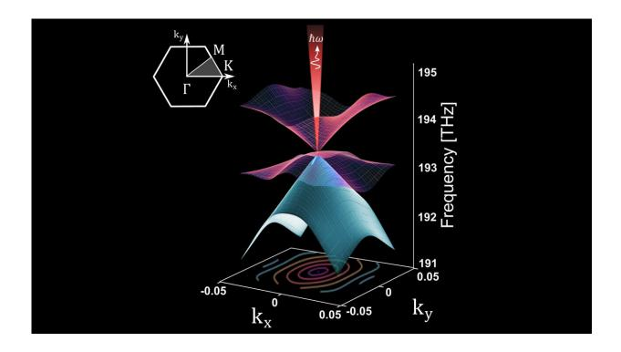
Schematic showing the "Dirac cones." Light is emitted synchronously from the entire semiconductor cavity as a result of the Dirac point singularity. Credit: the Boubacar Kanté group
