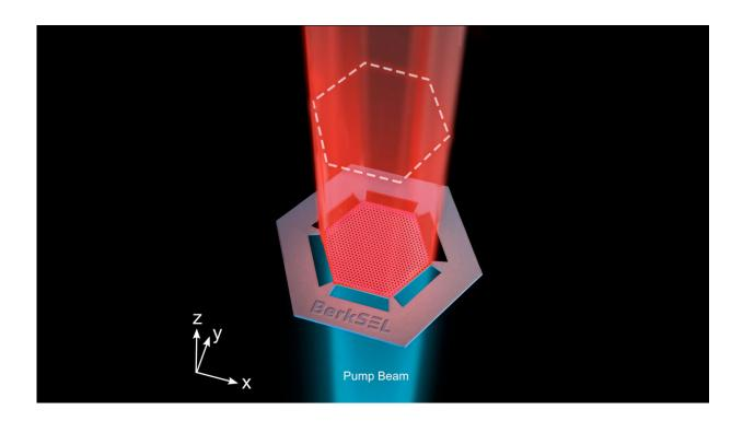
Schematic of the Berkeley Surface Emitting Laser (BerkSEL) illustrating the pump beam (blue) and the lasing beam (red). The unconventional design of the semiconductor membrane synchronizes all unit-cells (or resonators) in phase so that they are all participating in the lasing mode. Credit: the Boubacar Kanté group
