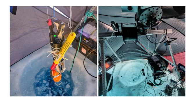
From inside a tent, Evans and Whelihan placed instruments such as profiling sensors (left) into 36-inch holes drilled through the ice. A mounting framework (right) supported the laboratory-developed fiber platform and a winch moving the profiling sensors. Credit: Massachusetts Institute of Technology
