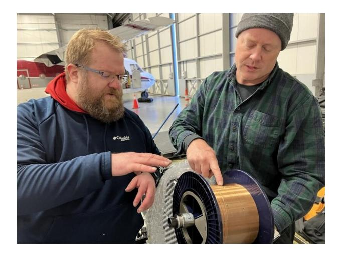
Lincoln Laboratory's Ben Evans (left) and Dave Whelihan deployed this spool — featuring 230 feet of polymer fiber with embedded temperature and depth sensors — in the Arctic. Credit: Seth Koenig/U.S. Navy
