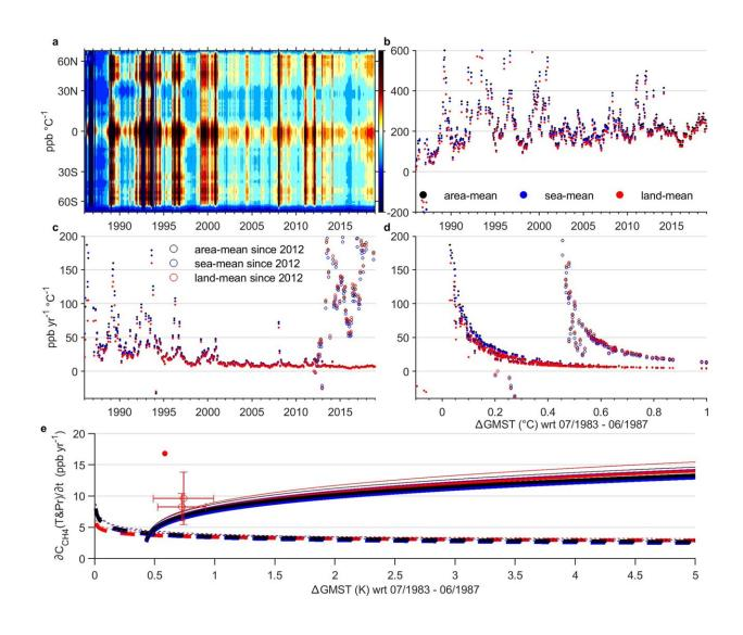
Methane-climate feedback sensitivities and projected annual mean climate-feedback-contributions. Sensitivities are expressed in ppb  $^{\circ}C^{-1}$  (a, b) or ppb yr $^{-1}$   $^{\circ}C^{-1}$  (c, d) vs time (a–c), latitudes (a), or just  $^{\circ}C$  (d). For (e), the projected annual mean  $\Delta C_{CH4}$ , climate/ $\Delta t$  curves are fitted based on values with both positive
