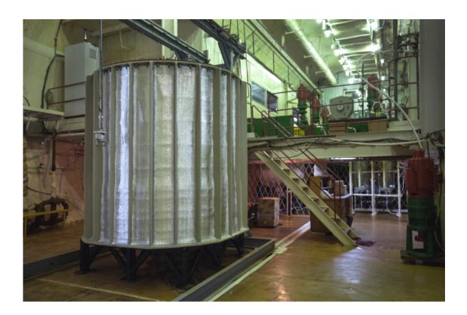
Located deep underground at the Baksan Neutrino Observatory in the Caucasus mountains in Russia, the completed two-zone gallium target, at left, contains an inner and outer tank of gallium, which is irradiated by an electron neutrino source. Credit: A. A. Shikhin
