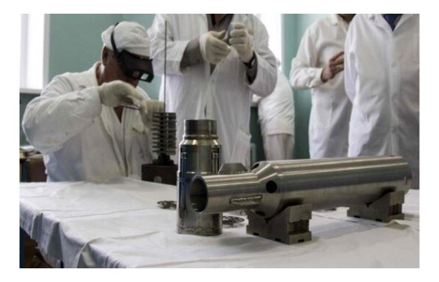
A set of 26 irradiated disks of chromium 51 are the source of electron neutrinos that react with gallium and produce germanium 71 at rates which can be measured against predicted rates. Credit: A. A. Shikhin
