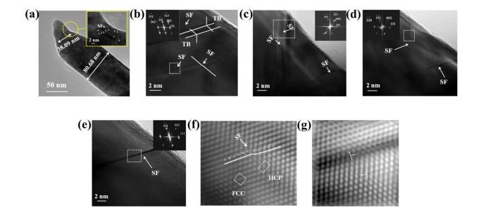
Figure 4. Microstructural characterization of different parts of a silver nanowire after fracture under film shear stress. Credit: Wang Mengjiao
