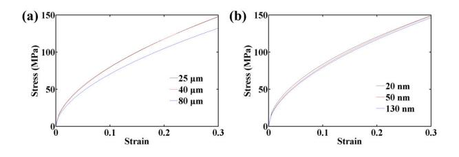
Figure 3. Stress-strain curves of silver nanowire films with different nanowire diameters and film thicknesses. Credit: Wang Mengjiao
