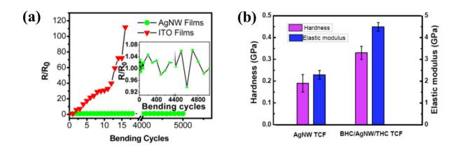
Figure 1. Bending resistance and surface scratch resistance of silver nanowire films for folding screens. Credit: Wang Mengjiao
