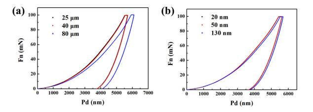
Figure 2. Load-displacement curves of silver nanowire films with different nanowire diameters and film thicknesses. Credit: Wang Mengjiao
