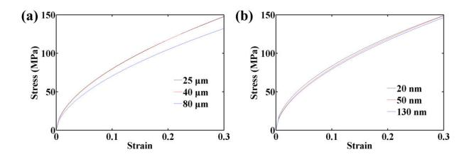
Figure 3. Stress-strain curves of silver nanowire films with different nanowire diameters and film thicknesses. Credit: Wang Mengjiao
