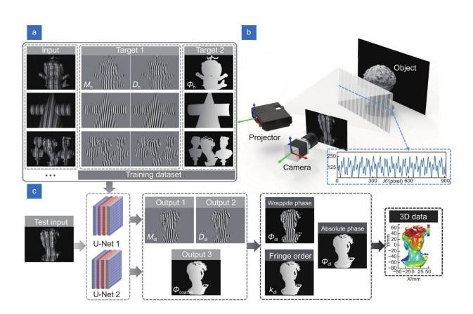
Flowchart of the proposed approach. (a) Part of network training data sets. (b) Hardware system and the cross-section intensity distribution of the designed composite fringe pattern. (c) Test data and prediction results obtained by the training model. Credit: *Opto-Electronic Advances* (2022). DOI: 10.29026/oea.2022.210021
