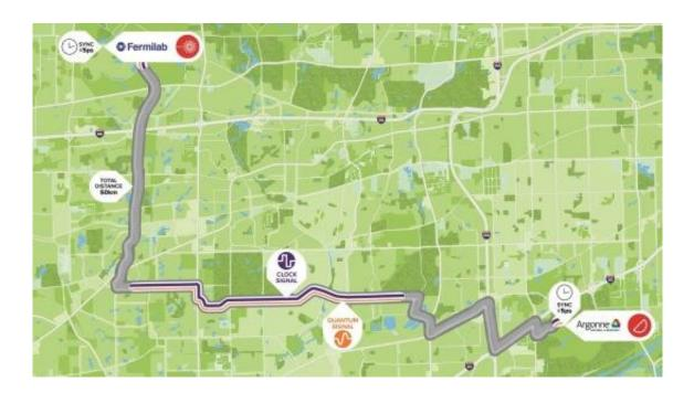
To test the synchronicity of two clocks — one at Argonne and one at Fermilab — scientists transmitted a traditional clock signal (blue) and a quantum signal (orange) simultaneously between the two clocks. The signals were sent over the Illinois Express Quantum Network. Researchers found that the two clocks remained synchronized within a time window smaller than 5 picoseconds, or 5 trillionths of a second. Credit: Lee Turman, Argonne National Laboratory
