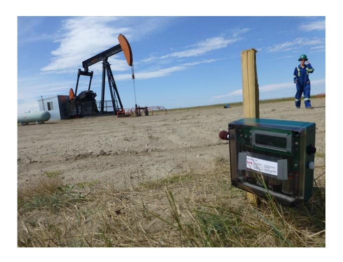
An autonomous recording unit used to determine how constant pumpjack noise varies with changing weather conditions. Credit: Colin R Swider, Author provided
