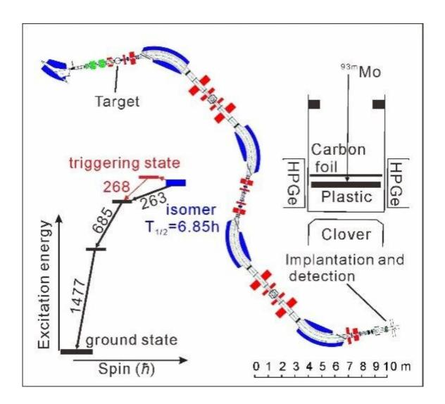
Experimental setup in the present work. The secondary beam line RIBLL is shown with the corresponding distance scale. In the lower left area, the isomer depletion of <sup>93m</sup>Mo is sketched together with the spontaneous decay of the long-lived isomer. The setup for implantation and detection is shown in the upper right area. Credit: *Physical Review Letters* (2022). DOI:
