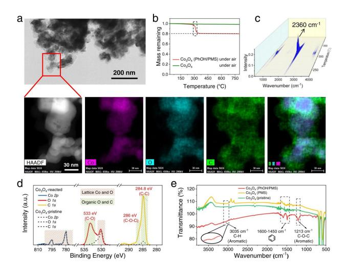
Product analyses of the model reaction system ( $Co_3O_4$ /PMS/PhOH). a STEM, HAADF, and EDS elemental mapping images of the  $Co_3O_4$  after the reaction. b TGA curves of the pristine and reacted  $Co_3O_4$  in air ( $O_2$ ). The mass loss of 20% for the reacted  $Co_3O_4$  was equal to the initial concentration ratio of [PhOH] to [PhOH] + [ $Co_3O_4$ ], which indicates that the pollutant molecules were fully
