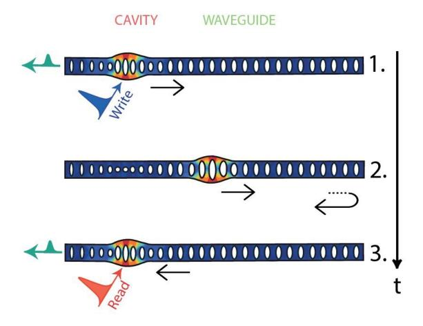
Sketch summarising the creation of (1) a traveling single phonon inside a waveguide (2), which can then be detected (3) after reflecting off the end of the waveguide. Credit: Gröblacher Lab, TU Delft.
