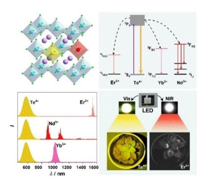
Schematic of efficient NIR luminescence in Te<sup>4+</sup>/Ln<sup>3+</sup> co-doped Cs<sub>2</sub>ZrCl<sub>6</sub> microcrystals. Credit: Prof. CHEN's group
